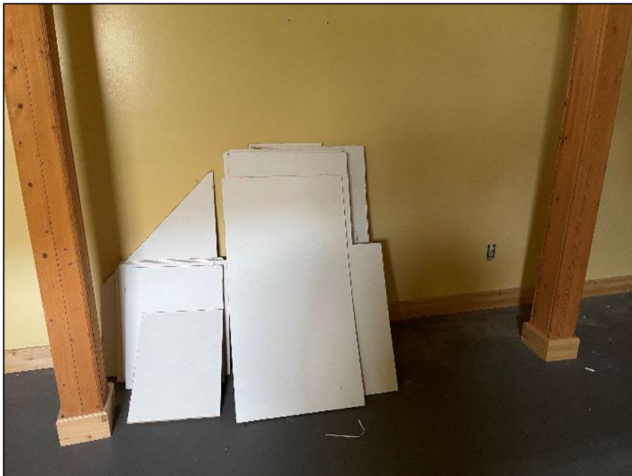
PHOTOGRAPH #12: Ceiling Tile - Basement Living Room (2x4) (Non-Asbestos)
