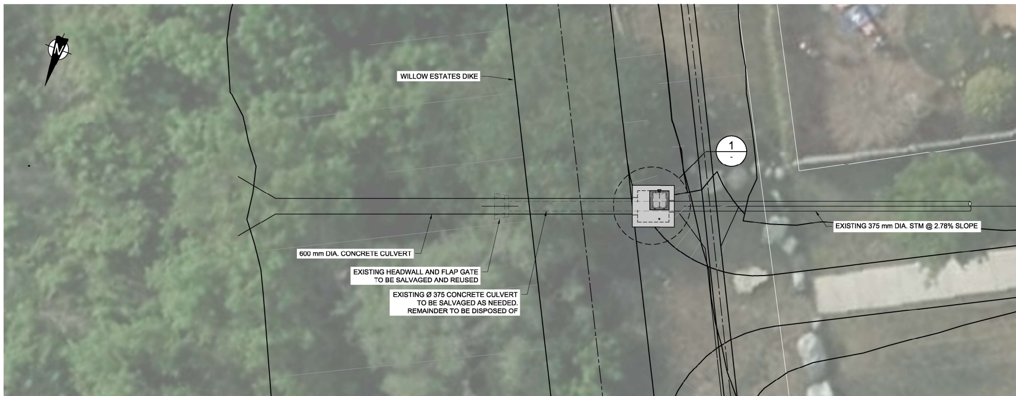
PLAN - CULVERT UPGRADE AT STA 1+246 Scale 1:75
