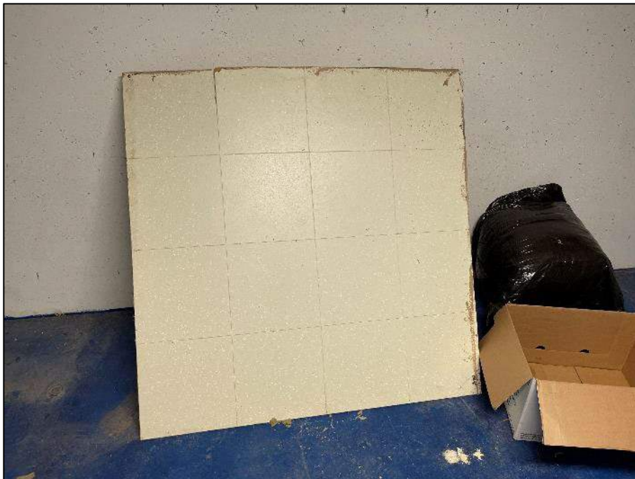
PHOTOGRAPH #10: Ceiling Tile - Basement (Non-Asbestos)
