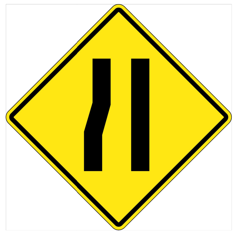
ROAD NARROWS FROM LEFT WA-23-T
